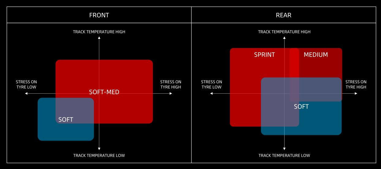
The stress that is put on a tyre, and by consequence impacts its performance and durability, is a combination of different factors such as track layout, surface roughness (µ), rider skill, type of motorcycle...
